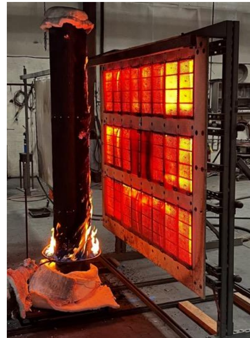
FR Wrap Fire Test on Utility Poles
