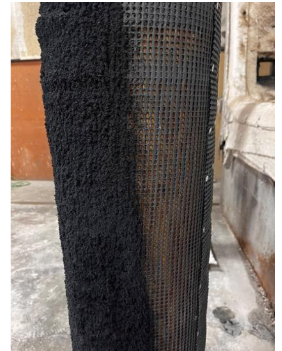
FR Wrap Fire Test on Utility Poles
