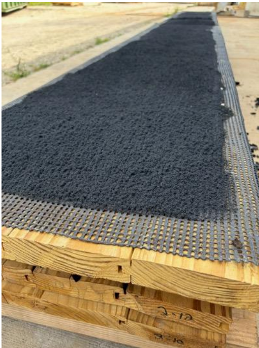
FR Wrap Fire Test on Dimensional Lumber
