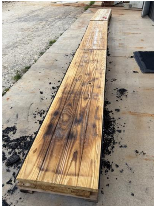
FR Wrap Fire Test on Dimensional Lumber
